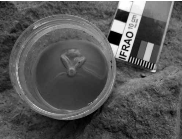
Fig. 6 - Colour obtained from pigment No. 8 and mixed with binder (Banyan tree leaves' milk).
