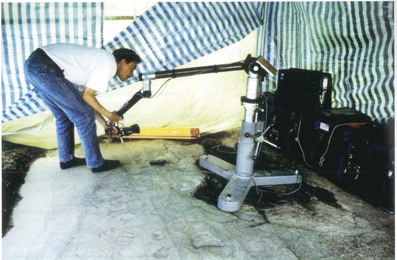
Fig. 2. Testing the NOMAD laser scanner at rock no. 151, Tanum, Sweden.
