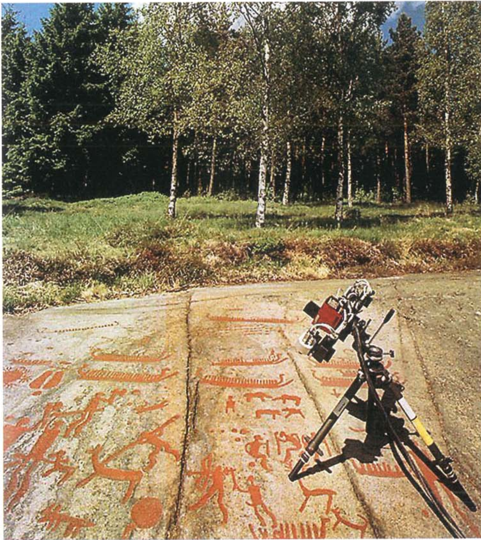
Fig. 3. Testing the ATOS video scanner system in field conditions.
